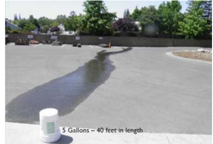
Five gallon spill on sloped surface
