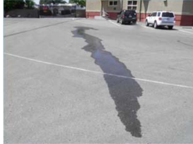
Two gallon spill on sloped surface
